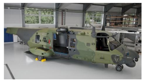
Fig. 5: The first training rig has been completed and delivered to the German Air Force Training Academy in Fassberg. Four additional models will follow.
