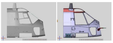
Fig. 2: The three-dimensional scan data (left) is imported as an STL mesh to CAD systems for reconstruction (right). Simulations are also carried out on the basis of FEM computations.
