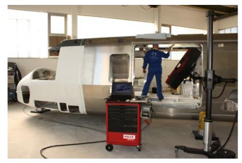
Fig. 3: During final assembly of the training rigs, more 3D measurements are carried out with ATOS Triple Scan. The correct positioning of the individual components is also verified point-to-point using an optically tracked touch probe.
