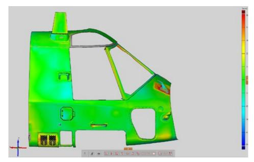
Fig. 4: During final assembly of the training rigs, the outer shell or "skin" is inspected for possible deformations. The full-surface measurement data is compared with the CAD data set. Deviations from CAD are highlighted in color and easily recognizable as problematic areas, enabling specific improvements to be made to the manufacturing process.
